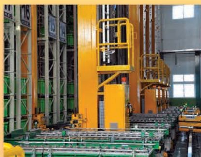
▼自動倉庫 Computer Warehousing
